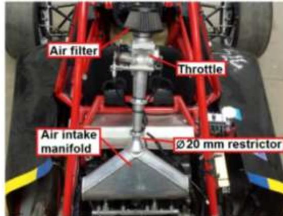
Fig1. Manifold with Ø20mm air restrictor.
