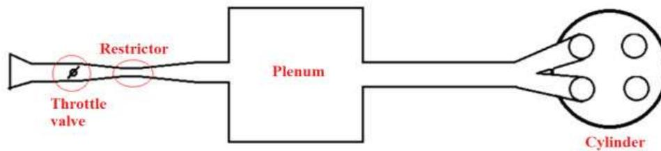
Fig.(3) Assembly of intake system [9]
