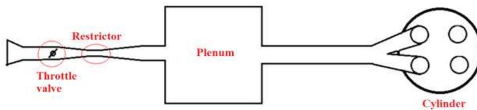
Fig.(3) Assembly of intake system [9]
