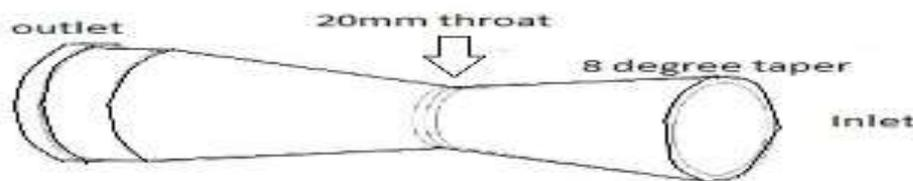
Fig (2). Basic Design of Intake Restrictor
