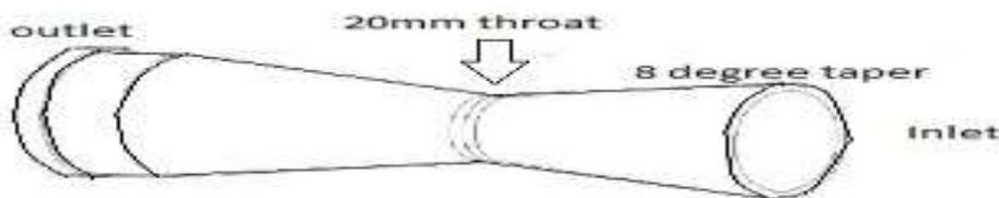
Fig (2). Basic Design of Intake Restrictor
